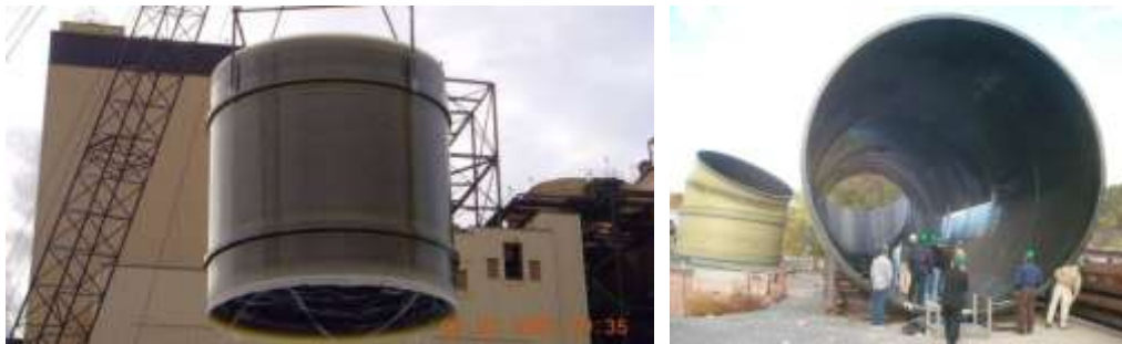
Figure 7. Large diameter FRP chimney flue liner, a) a module liner section and b) connection elbow (Rider, 2009)
