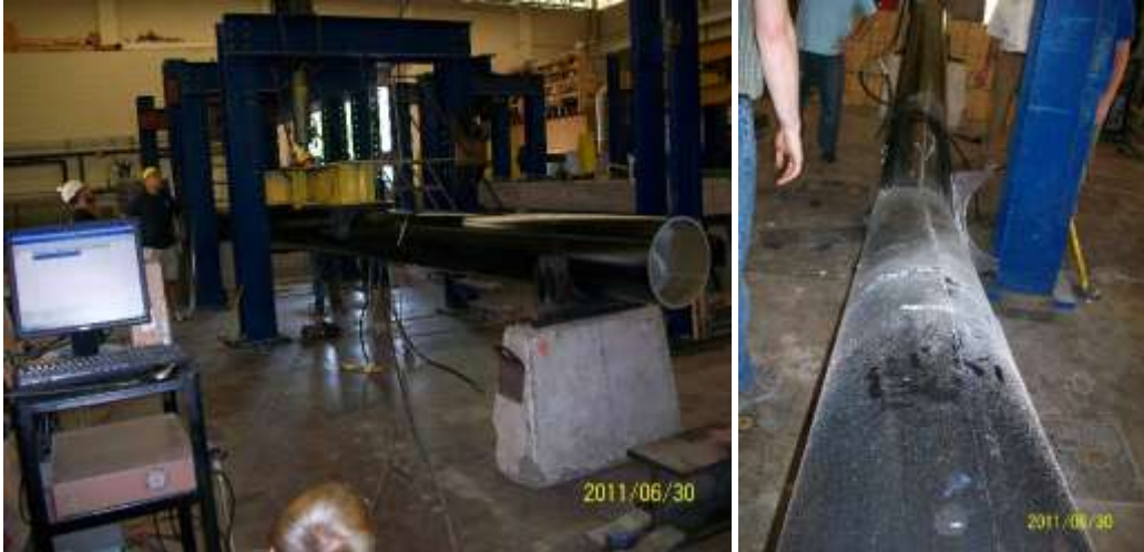
Figure 5. 16 inch diameter FRP pipe being tested at WVU-CFC laboratory (2011)
