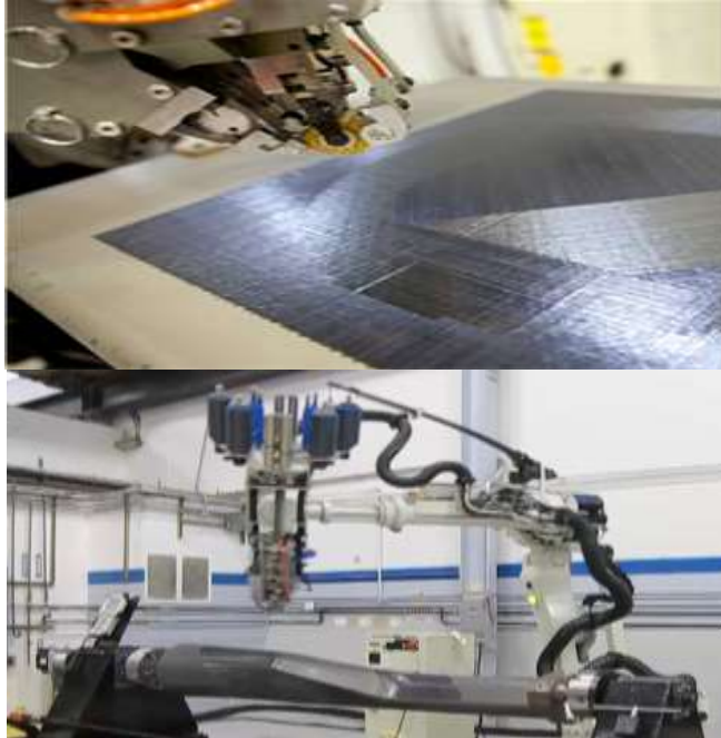
Figure 14: Additive manufacturing of advanced composite materials part, with automatic fiber placement (Cormier, 2016)
