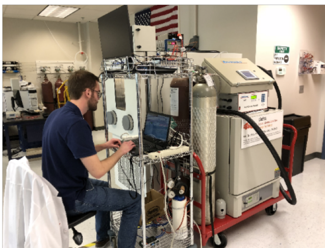
Figure 4 Component level testing in an environmental chamber at the DADSS Lab in Marlborough, MA
